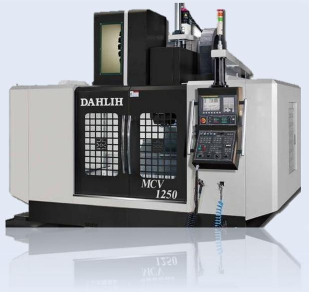
Heavy Duty Vertical Machining Centre with Box Guideways
